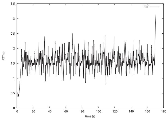
Fig. 13. RTT corresponding to FTP transfer with Motorola handset.
