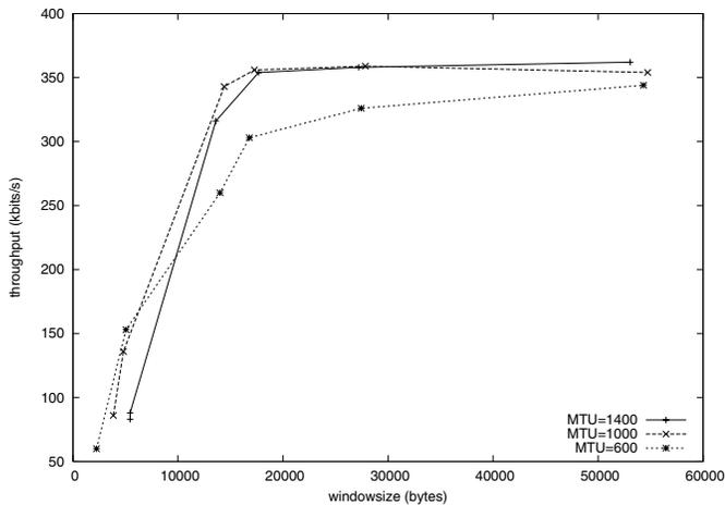
Fig. 5. Throughput as a function of window size for various MTU values.
