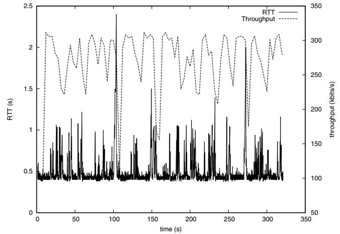
Fig. 1. RTT and throughput during an FTP transfer in a moving car, with two handovers visible at around  $t = 100$  s and  $t = 270$  s.
