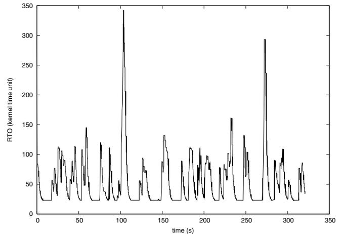
Fig. 2. The TCP RTO threshold during the FTP transfer in a moving car.
