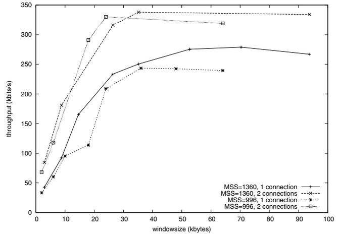
Fig. 6. Throughput as a function of window size for various MSS values, using one or two parallel connections.
