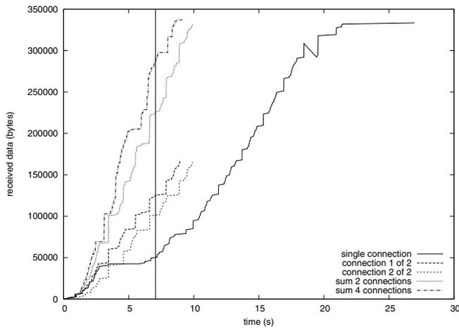
Fig. 4. The amount of received data as a function of time during download of a web page using varying number of connections. The vertical line marks the shortest possible theoretical transfer time ignoring higher-layer protocol overhead.
