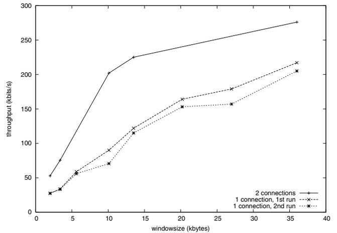
Fig. 7. Dependence of throughput on the window size for small MSS value, with one and two parallel connections. For illustration of the relatively high consistency of the UMTS channel, two individual runs of transfers using a single connection are shown.
