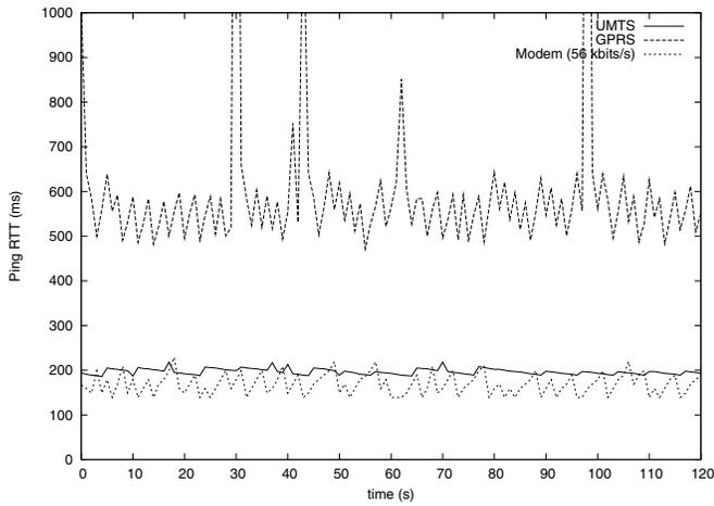
Fig. 3. The “raw” RTTs of UMTS, GSM and 56kbps modem channels as measured using ping.
