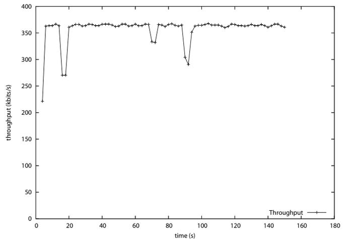
Fig. 10. Throughput during an FTP transfer as measured using Nokia handset.
