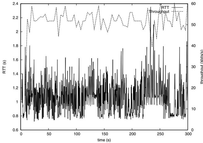
Fig. 8. The RTT and throughput during an FTP transfer between two mobile stations.
