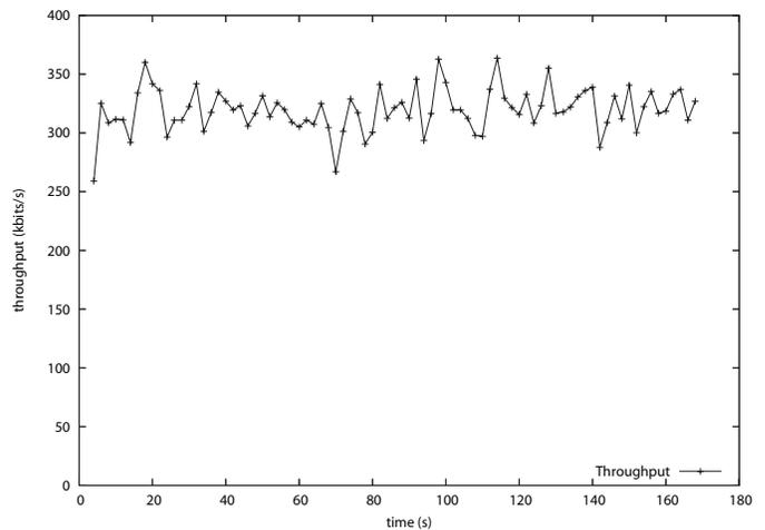
Fig. 11. Throughput during an FTP transfer using Motorola handset.
