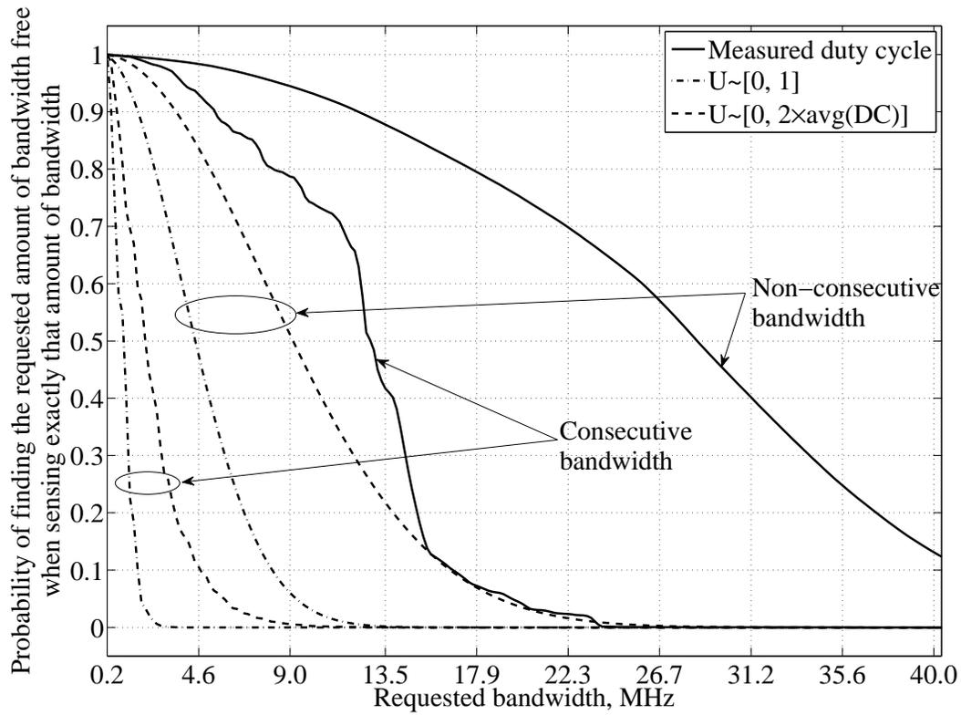
Fig. 3. Comparison between the duty cycle measured in the UMTS uplink band and artificial spectrum occupancy data generated based on the model described in [14].
