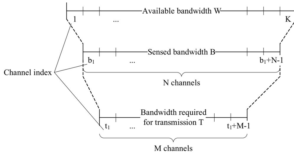
Fig. 4. Relations of the different bandwidths and numbers of channels used throughout the formulation of the tradeoff between the outage probability and the sensed bandwidth.
