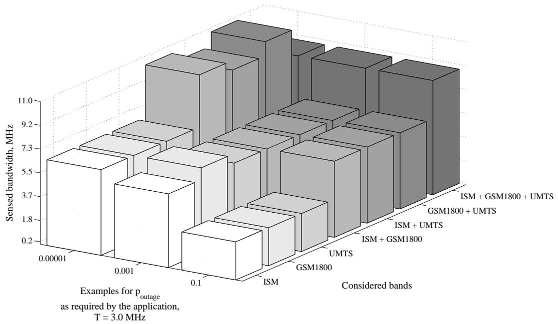
Fig. 8. Impact of sensed bandwidth  $B$  on the outage probability  $p_{outage}$  in several bands: ISM, GSM1800, UMTS, or combination of some bands: ISM + GSM1800, ISM + UMTS, GSM1800 + UMTS, ISM + GSM1800 + UMTS. Three target outage probabilities are considered:  $10^{-1}$  (voice quality),  $10^{-3}$ ,  $10^{-5}$ .
