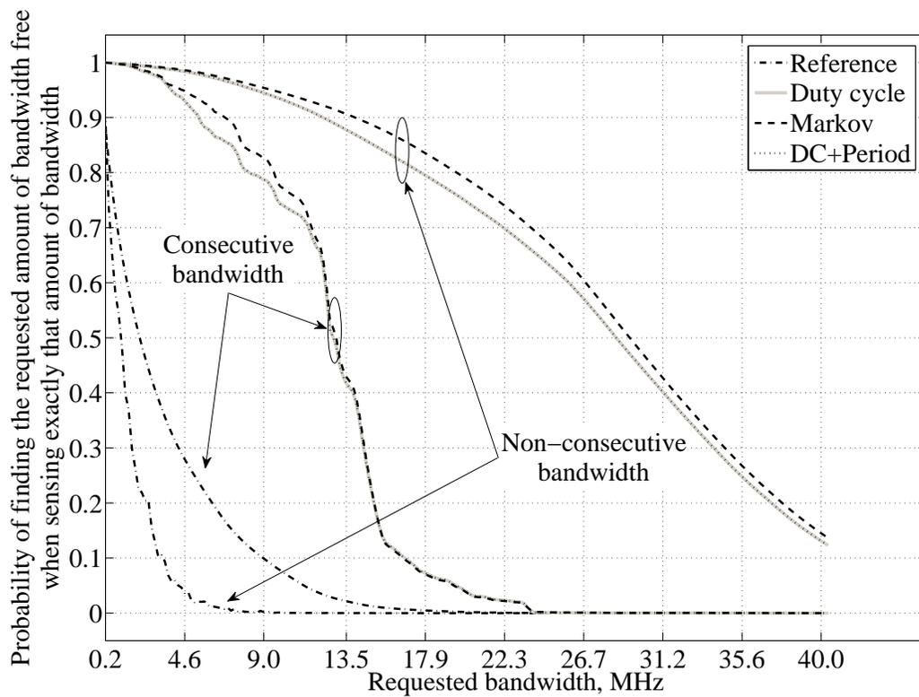
Fig. 1. Comparison of the four methods for adaptive spectrum sensing for the UMTS uplink band. The curves for duty cycle and DC+Period cannot be easily distinguished because of the negligible impact of periods and, thus, a very small difference between them.
