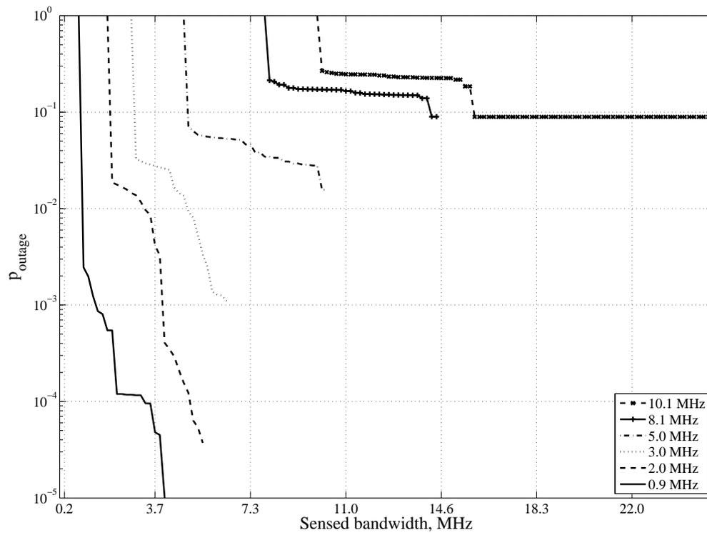
Fig. 7. Impact of sensed bandwidth  $B$  on the outage probability  $p_{outage}$  for the GSM1800 uplink band. Curves that stop reached 0 and cannot be represented in logarithmic scale anymore.
