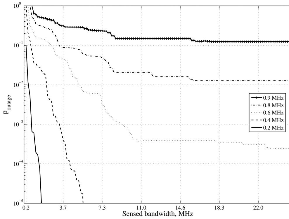
Fig. 6. Impact of sensed bandwidth  $B$  on the outage probability  $p_{outage}$  for the GSM uplink band.
