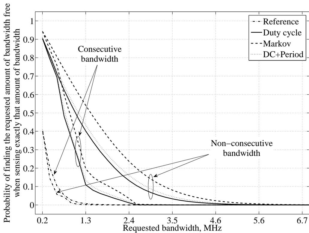
Fig. 2. Comparison of the four methods for adaptive spectrum sensing for the GSM uplink band.
