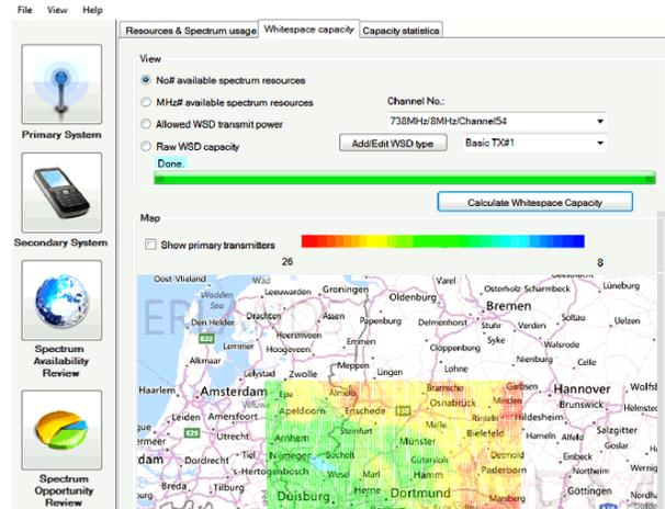
Figure 3. Screenshot of GUI, showing a heatmap result of calculated secondary network capacity and various configuration tabs.
