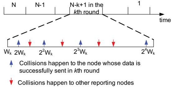
Fig. 1. An illustration of contention cycles. Each contention cycle has different collision probability due to different number of competing nodes.
