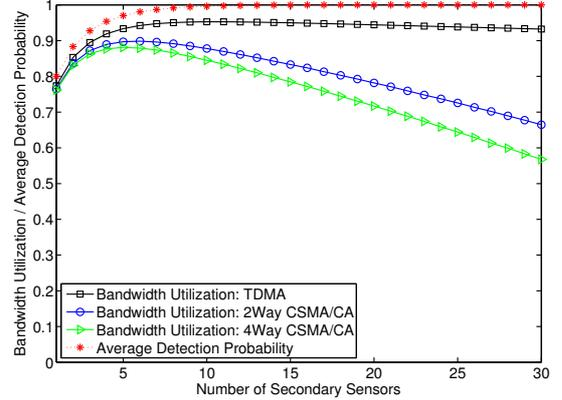
Fig. 3. A comparison of three multiple access schemes,  $m = 6$ ,  $P_d(1) = 0.8$ .
