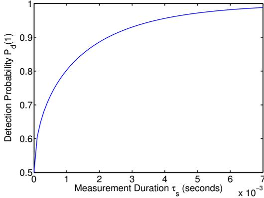
Fig. 2. The relationship between detection probability  $P_d(1)$  and spectrum measurement duration  $\tau_s$ .
