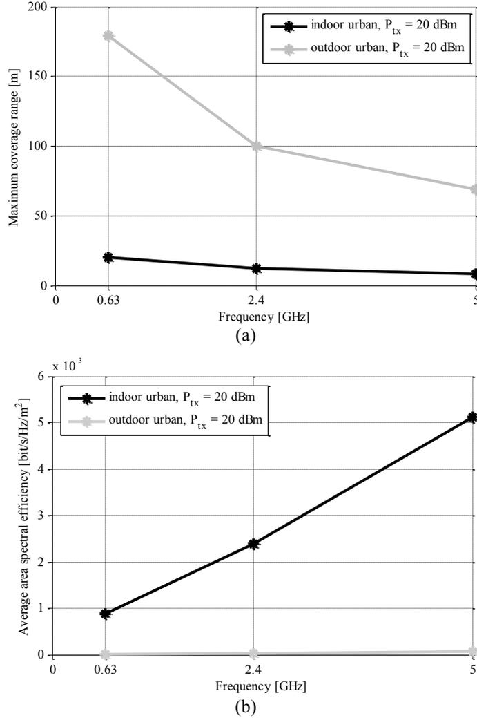
**Figure 3.** Slices out of the N-dimensional space analysis of a Wi-Fi-like wireless network operating in the outdoor urban and indoor urban scenarios, showing the effect of varying the centre operating frequency on: (a) maximum (cell-edge) AP coverage range and (b) average area spectral efficiency (average AP downlink rate normalized by the width of the channel occupied by the AP and the size of the AP’s coverage area).
