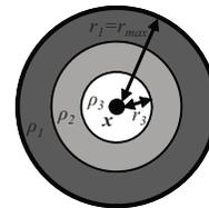
Fig. 3. Illustration of auto-rate function  $\rho(\beta)$ , whereby AP  $x$  provides a raw bit rate of  $\rho_n$  to a user located within a range of  $r_n$  (only showing up to  $n = 3$  for the sake of clarity); the maximum coverage range  $r_{max}$  corresponds to the boundary of the coverage area (cell) of AP  $x$ .
