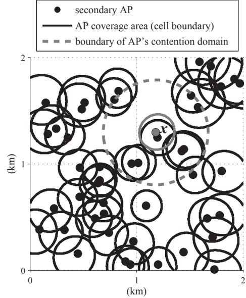
Fig. 4. Illustration of inter-AP interference (all APs co-channel, outdoor urban scenario with  $P_{tx} = 30$  dBm and 24 MHz channel in TVWS). As per CSMA/CA, the eight APs inside the contention domain of AP  $x$  reduce its channel access time to one ninth, whereas the remaining APs cause interference during its transmission (reducing the coverage range of AP  $x$  by decreasing the SINR of an associated user).
