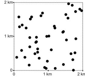
Fig. 1. Example secondary network realisation for the outdoor urban deployment scenario, showing random AP locations as generated using a Poisson point process with density  $\lambda = 12.5/\text{km}^2$ .
