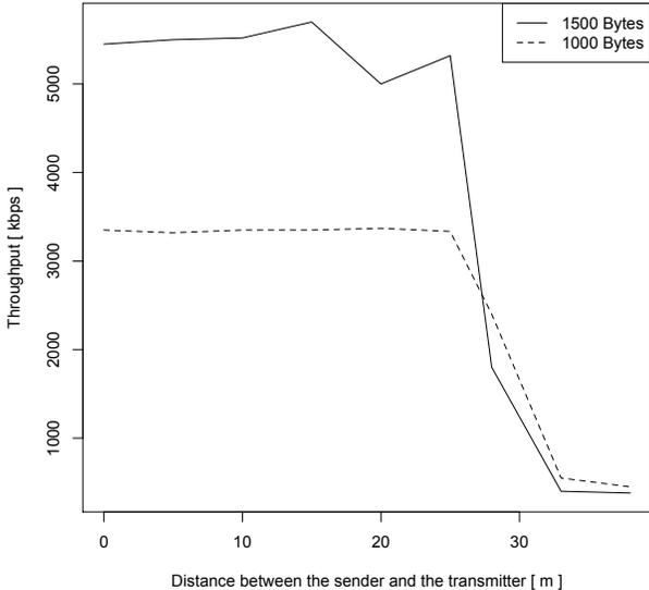
**Figure 1: Throughput of a UDP connection over a IEEE 802.11b Wi-Fi link as a function of distance between the transmitter and the receiver for two different frame sizes.**
