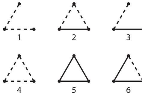
**Figure 8: The three-node network motifs occurring in the Outdoor Wi-Fi scenario. Solid lines denote edges of type one, and dashed lines edges of type two.**
