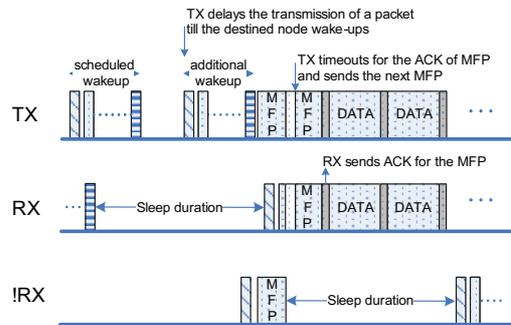
Fig. 4. Unicast transmission for SA-MAC, where neighbourhood sleep schedule information is combined with preamble strobing technique. After an MFP is acknowledged, data frame(s) are immediately sent.
