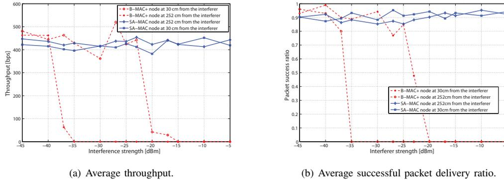
Fig. 10. Throughput and successful packet delivery ratio achieved for B-MAC+ and SA-MAC in the presence of an interferer at asymmetrical distance from the nodes. All the nodes used the rate of 0.5 packet/second and operated at the sampling period of 1s with radio transmit power of -15dBm. The two B-MAC+ and SA-MAC nodes were placed at a distance of 282 cm from each other.
