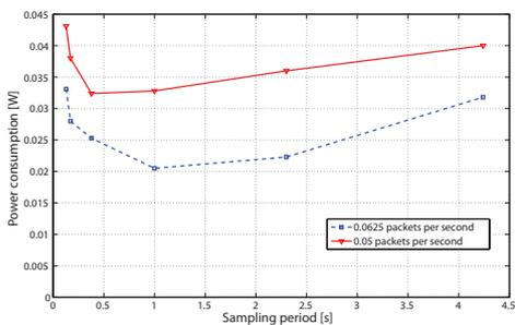
Fig. 6. Power consumption of a node at different sampling periods. In these measurements, a small non-congested network of three TelosB nodes is considered. The nodes use four channels and are in the perfect wireless range of each other with 0dBm of transmit power.
