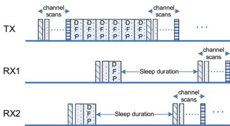
Fig. 3. Broadcast transmission in SA-MAC. Back-to-back DFPs are sent for a duration equal to the periodic channel check interval. The data bytes are piggybacked onto the preamble frames.
