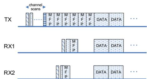
Fig. 2. Broadcast transmission in SA-MAC. Back-to-back MFPs are sent for a duration equal to the periodic channel check interval followed by the data frames.
