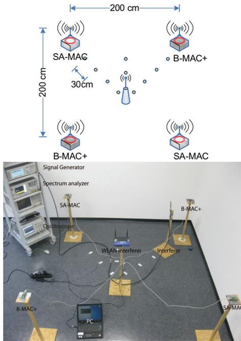
Fig. 8. Experimental setup for studying the co-existence behaviour and performance of B-MAC+ and SA-MAC in the presence of interference. The parameters altered during the experiments include the transmit power of sensor nodes, the spatial position and the strength of the interferer.
