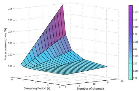
Fig. 7. Relationship of power consumption with the number of channels in the pool and the sampling period on TelosB platform during the low power listening operation.
