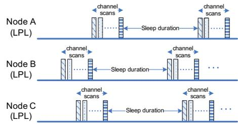
Fig. 1. Preamble sampling operation in SA-MAC protocol.
