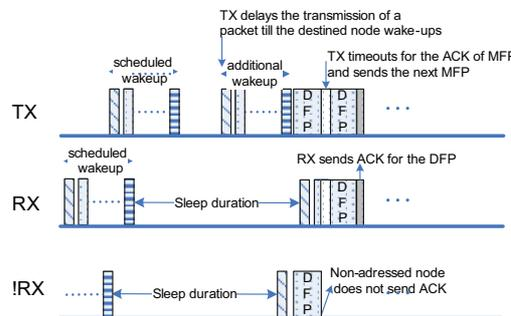
Fig. 5. Unicast transmission for SA-MAC. After a DFP is acknowledged, the transmitter stops sending further DFPs.
