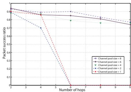
Fig. 12. Packet success ratio over multiple hops in the presence of non-uniform interferences at the two end of the networks. The transmit power of the nodes is set to be -15dBm and packet size used is 50 bytes.
