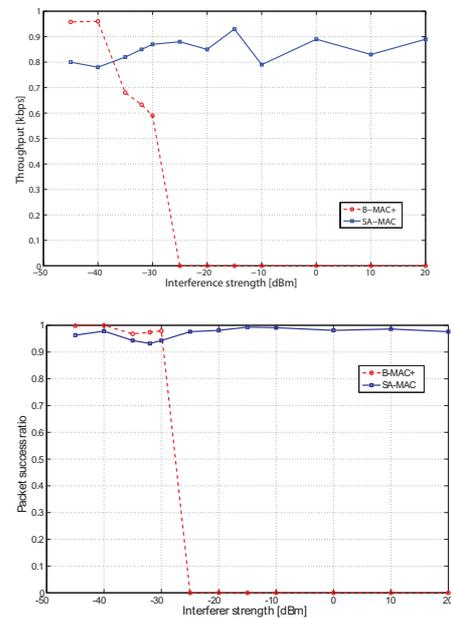
Fig. 9. Aggregate throughput (top) and successful packet delivery ratio (bottom) achieved for B-MAC+ and SA-MAC in the presence of an interferer at equidistant from the nodes. All the nodes transmitted a packet size of 100 bytes at the rate of 0.5 packets/second and operated at a sampling period of 1s with radio transmit power of 0 dBm. The two B-MAC+ and SA-MAC nodes were placed at a distance of 282 cm from each other.
