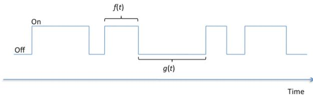
Figure 2. Semi-Markov ON/OFF channel model.
