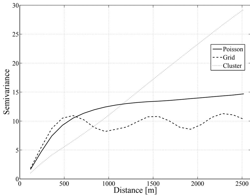
Figure 5: Impact of the underlying point process on the semivariogram based on system parameters configured to resemble a GSM network.
