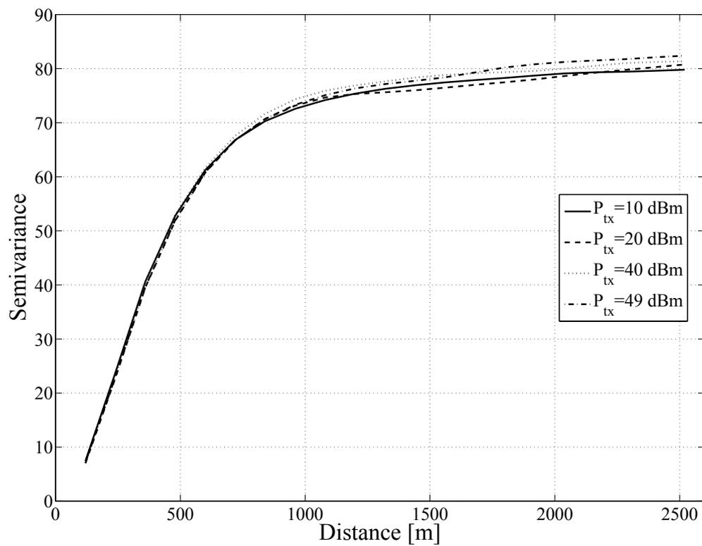
Figure 7: Impact of the simulated transmit power on the semivariogram based on further system parameters configured to resemble a GSM network.
