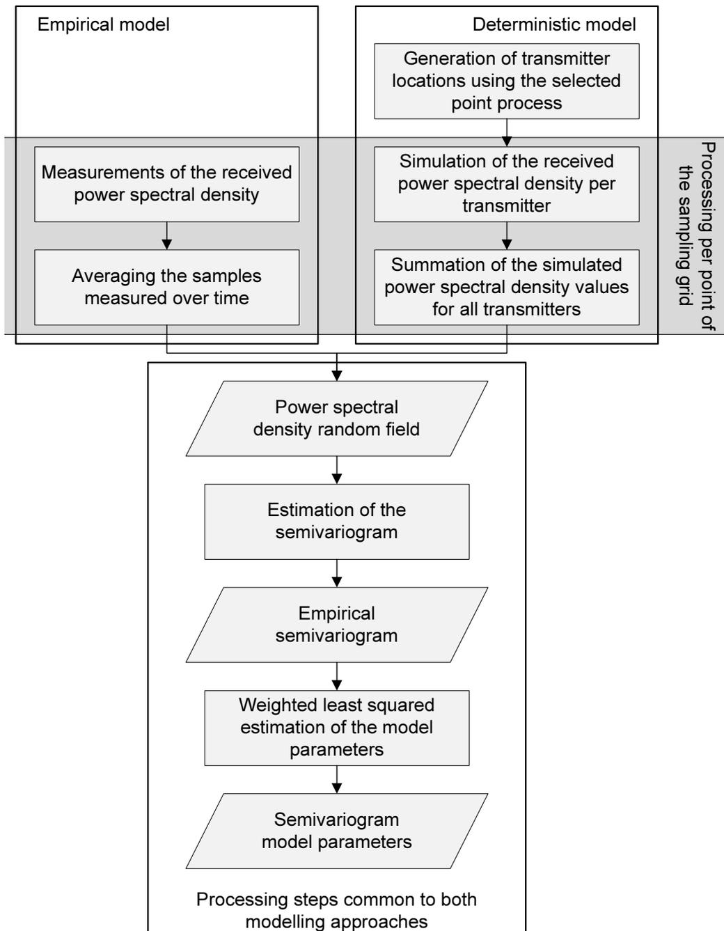
Figure 4: Flowchart of the different processing steps required to extract model parameters using either the empirical or the deterministic approach.
