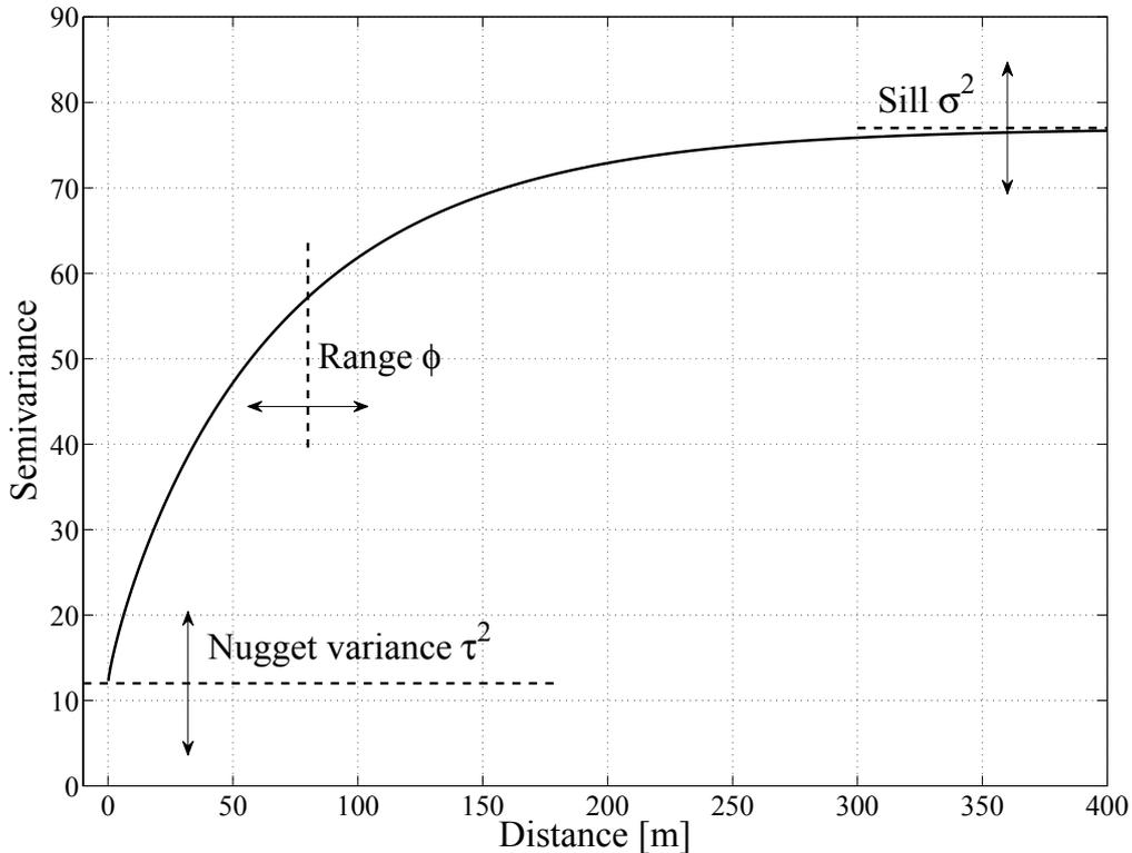
Figure 1: Meaning of the semivariogram model parameters and their impact on the shape of the semivariogram based on the example of the Matérn model.
