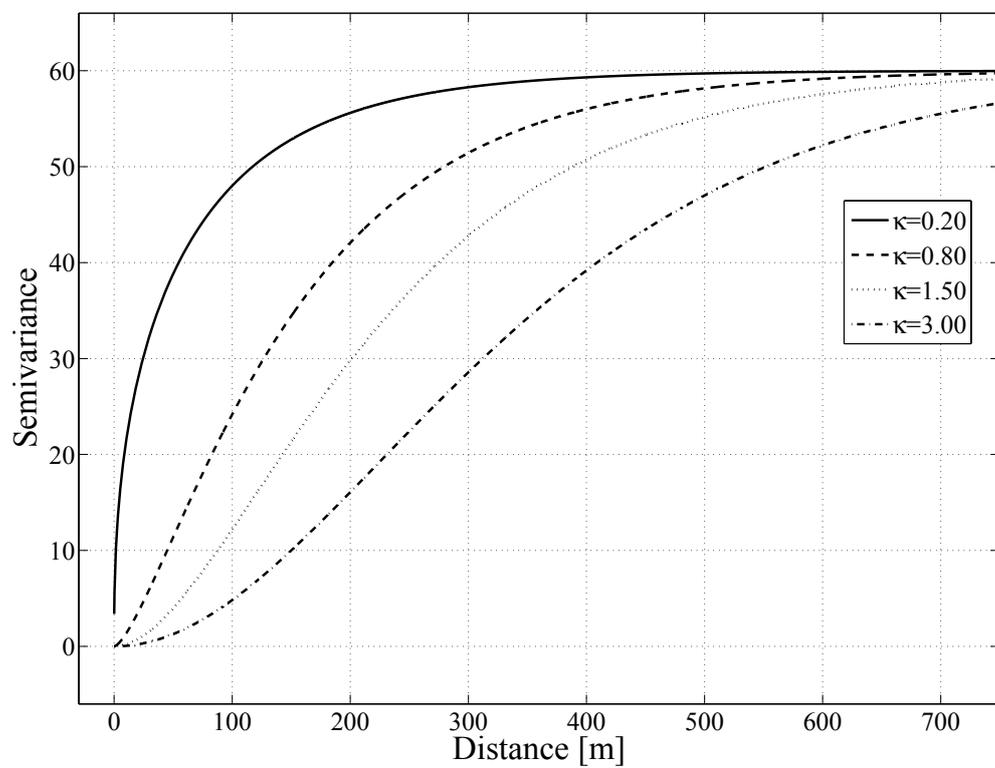
Figure 3: Comparison of different values for the parameter  $\kappa$  of the Matérn model on the shape of the semivariogram.
