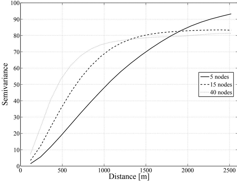
Figure 8: Impact of the node density on the semivariogram based on system parameters configured to resemble a GSM network.
