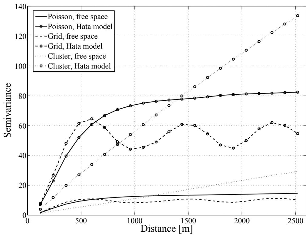
Figure 6: Impact of the propagation model on the semivariogram based on system parameters configured to resemble a GSM network.
