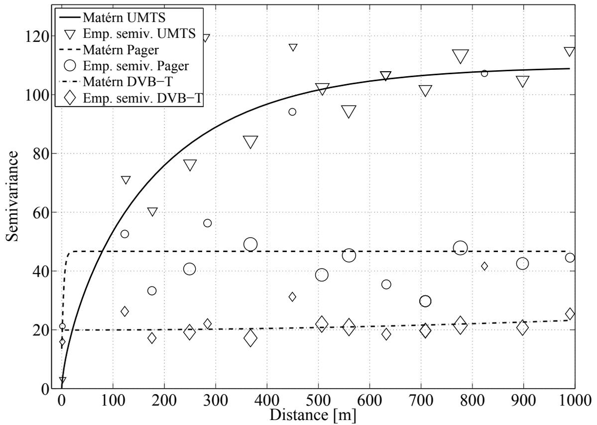
Figure 9: Fitted semivariograms based on the Matérn-model and estimated empirical semivariograms for the UMTS DL (5 MHz per channel, average over five channels at frequencies  $f \in [2110, 2170]$  MHz), a pager-service (200 kHz bandwidth at  $f = 466$  MHz), and DVB-T (6 MHz bandwidth per channel, average over three channels at  $f_1 = 490$  MHz,  $f_2 = 498$  MHz, and  $f_3 = 514$  MHz).
