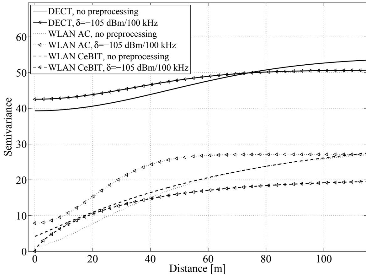
Figure 10: Fitted semivariograms based on the Matérn-model for the unchanged and the preprocessed input data sets for DECT networks ( $\approx 1.7$  MHz bandwidth per channel, average over ten channels at frequencies  $f \in [1880, 1900]$  MHz) and the WLAN system (20 MHz bandwidth per channel, average over the most popular channels 1, 6, and 11 in the 2.4 GHz ISM-band).
