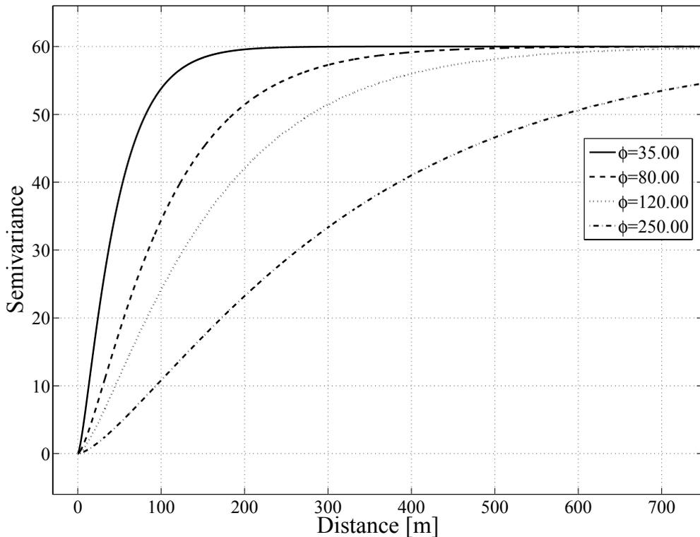
Figure 2: Comparison of different values for the parameter  $\phi$  of the Matérn model on the shape of the semivariogram.
