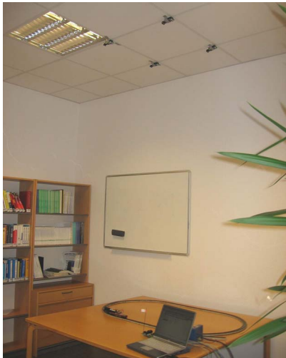
Figure 4: Experimental setup for measuring positioning accuracy of a moving object. Listening nodes are mounted on the ceiling, a beacon node is placed on the locomotive, while the gateway node is attached to the laptop.
